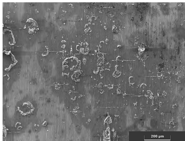
Fig. 3. SEM image of a sample exposed for 15 min illustrates the general pattern of crack embryos, noting that all cracks were initiated under salt particles.
