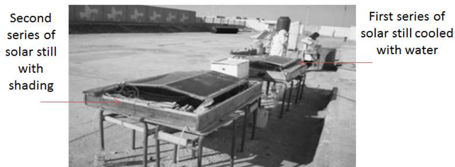
Figure 32: Zeroual's solar still [82]
