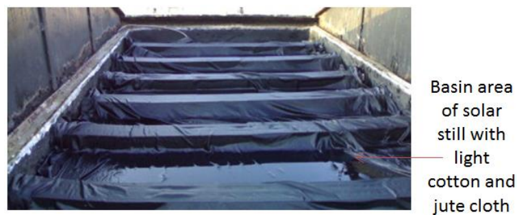
Figure 31: Photograph of the still with aluminium fin covered with black cloth in the basin [81]
