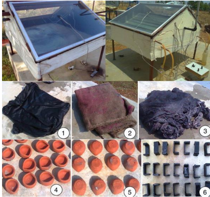
Figure 78: Double basin double slope and single basin single slope stills with (1) Black cotton cloth (2) Jute cloth (3) Waste cotton pieces (4) Clay pot- facing up (5) Clay pot- facing down (6) Mild steel pieces [231]
