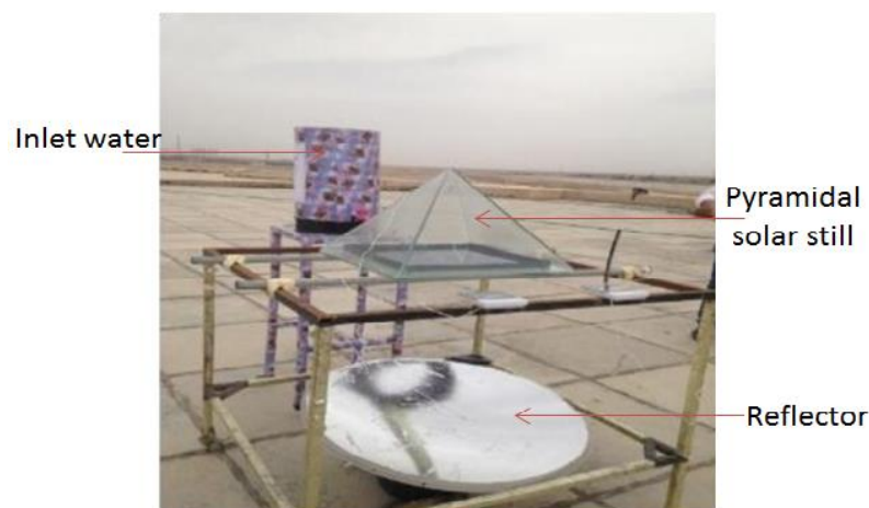
Figure 49: Pyramidal solar still with external reflector [99]
