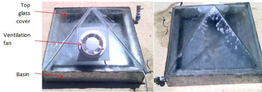
Figure 44: triangular solar still with fan to decrease the temperature of inner face of glasses [94]
