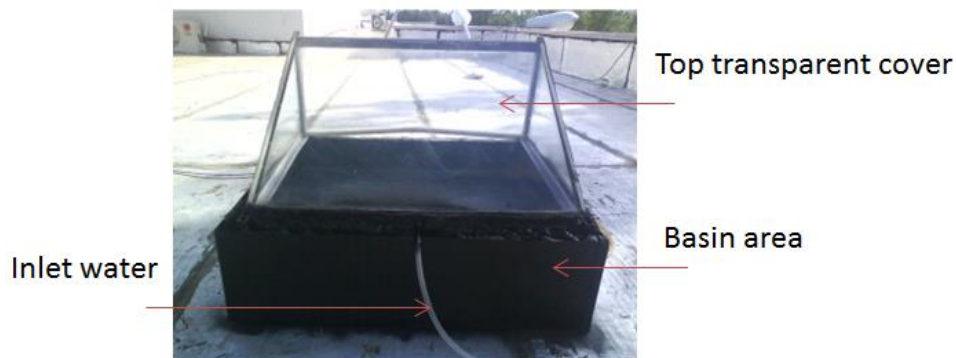
Figure 29: Tabrizi's double slope solar still tested with sand [79]
