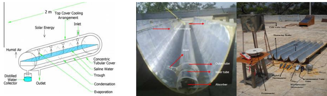
Figure 54: T. Arunkumar tubular solar still [104]
