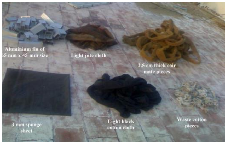
Figure 79 basin different basin wick material was used by Murugavel and Srithar [232]
