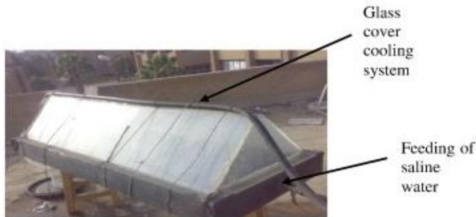
Figure 40: The double slope solar still with glass cover cooling [90]
