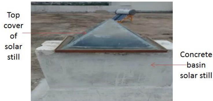
Figure 48: Kumar's pyramidal shape solar still [98]
