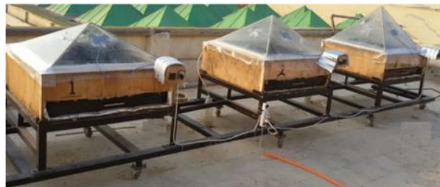
Figure 46: Three square pyramids solar still with three inclined angle [96]
