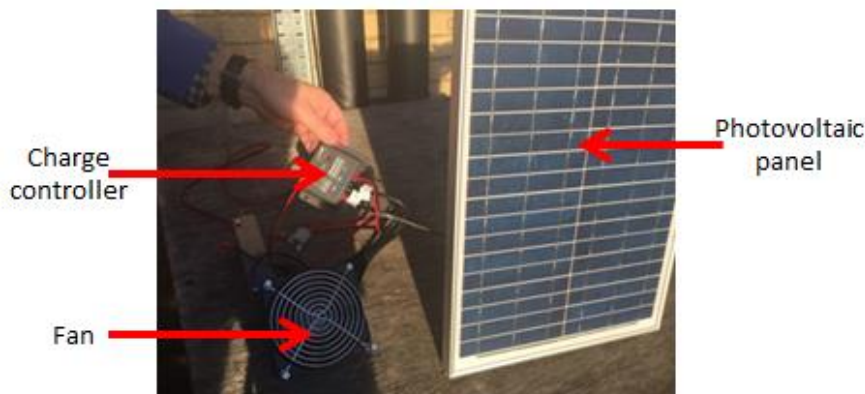
Figure 117: Testing the fan with the photovoltaic panel.
