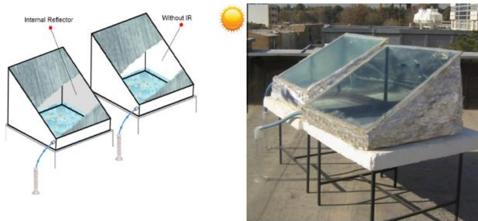
Figure 72: Karimi's single slope solar still with internal reflectors [205]
