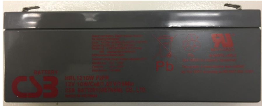
Figure 139: HRL 1210W DC battery
