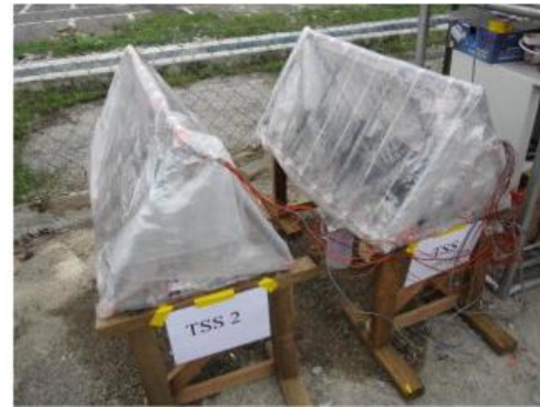
Figure 38: double slope solar still with waste material [88]
