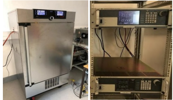
Fig. 1. Battery test equipment: (left) climate chamber, (right) power supply
