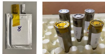
Fig. 2. LFP pouch cell (left) and NCA cylindrical cells (right) used in experiments
