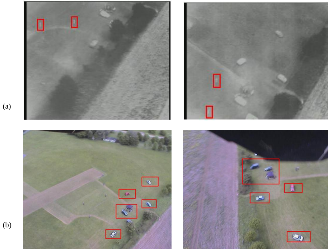
Figure 8. People detection results in thermal imagery (a) with optical images of the same scene with vehicle detections (b) (summer conditions).
