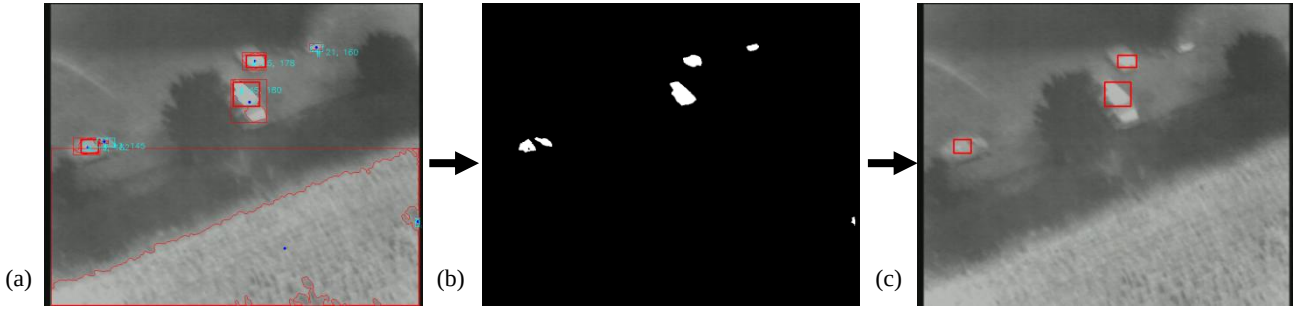
Figure 5. Thermal imagery with identified high intensity and contrast thermal signatures.
