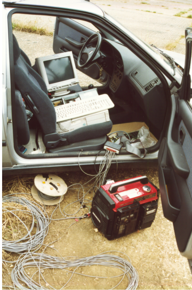
Figure 5.6: Computer, 15-pin connector interface box, cables and power generator used for the wind data measurements
