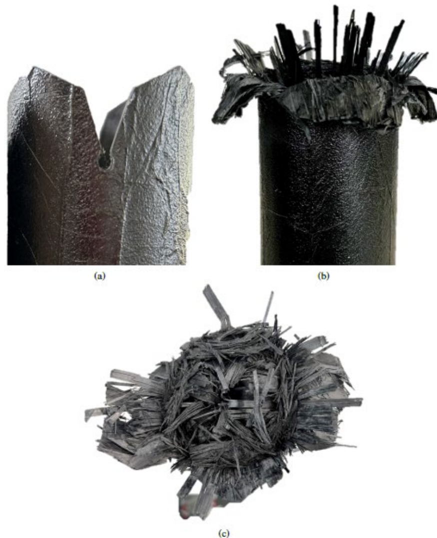
Figure 7. Illustration of the crushing deformation of the tested crown-tulip trigger (a), showing the petal formation with progressive peeling due to mode 1 delamination (b) and top view (c) of the crushed tube with visible debris wedges and internal petal formation.
