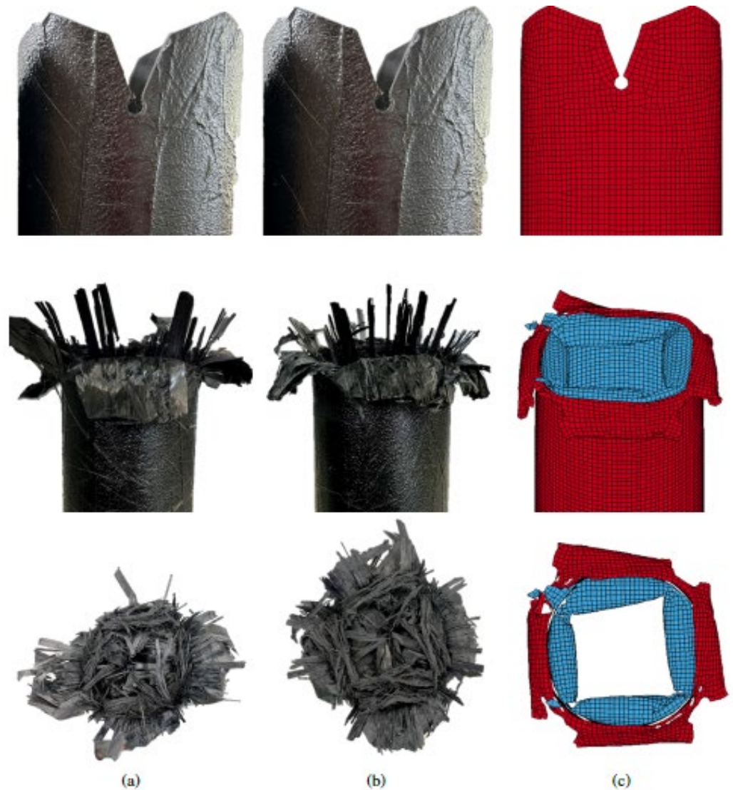
Figure 15. Comparison of 4T140°-20°-20 mm-Ø5 mm crown-tulip trigger deformation between physical test specimens T23147-Test A (a), T23148-Test B (b), and numerical model (c).
