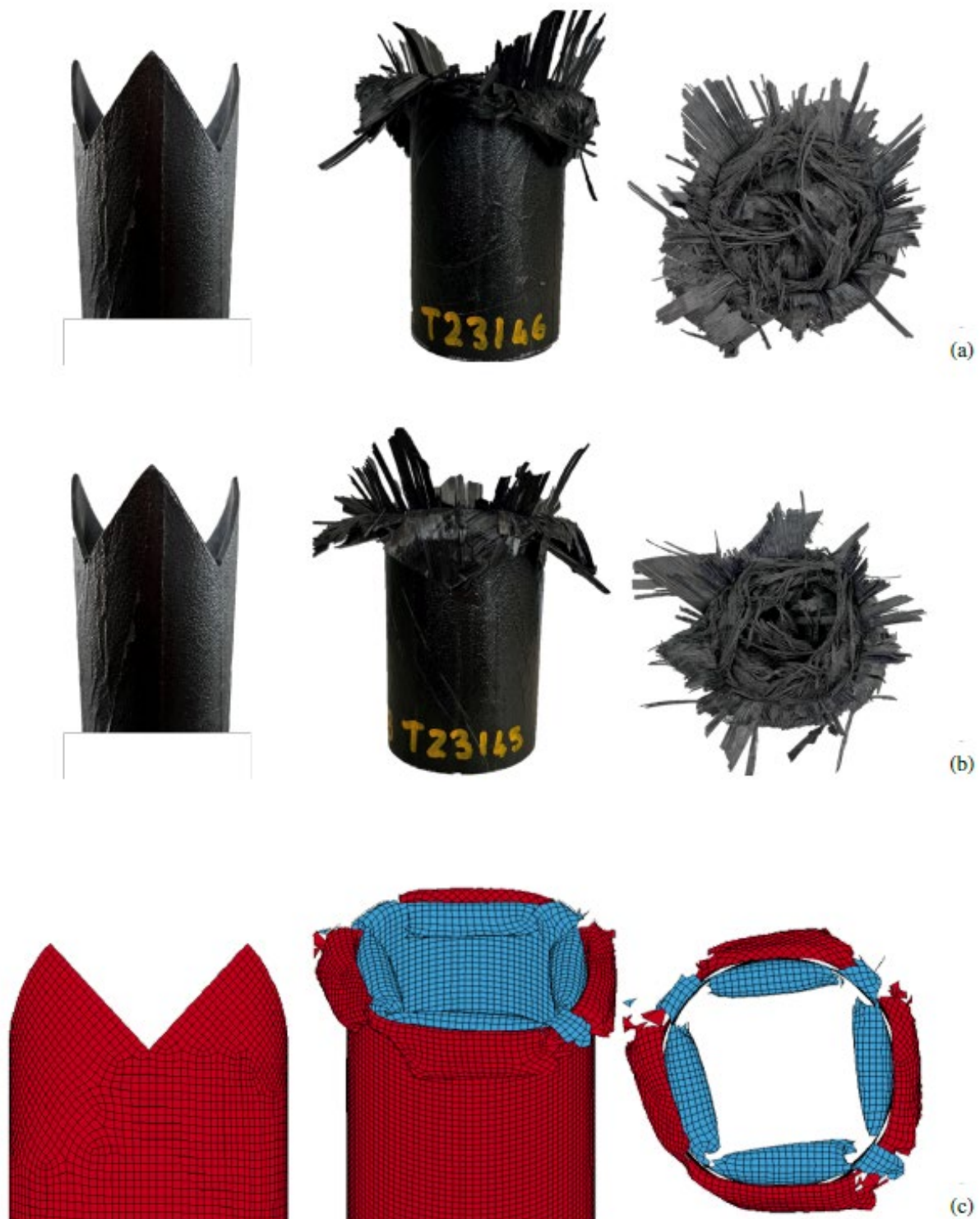
Figure 12. Comparison of 4T90° tulip trigger deformation between physical test specimens T23146-Test A (a), T23145-Test B (b), and numerical model (c).
