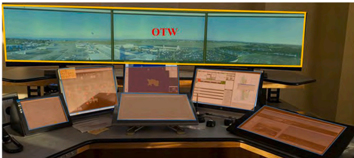
Fig. 3. The layout of digital tower module including seven components. The panorama displays (AOI-OTW) consisted with three screens to accommodate stitching images from 13 cameras for 240° filed-of-view on the airfield. The other six displays below OTW are exactly the same with physical tower module.
