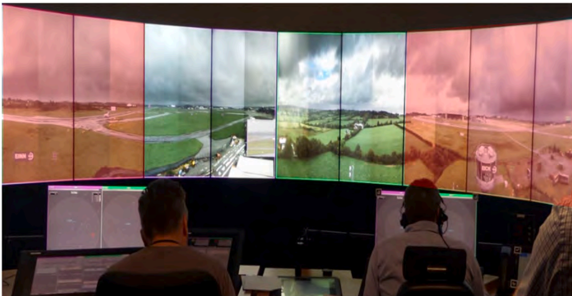
Fig. 1. The visual effects of distortions (shadowed by red) on both edges of OTW on digital tower module. The straight-line runway has been distorted to curved-shape due to the visual presentation of pan-tilt-zoom camera and panoramic displays.
