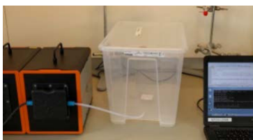
Fig. 2 Sampling of analyte from the box (middle) into the Crim-Track sniffer device (left). The experiment(s) were performed by using a laptop (right).
