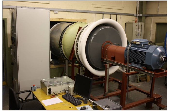
Fig. 5. PWG test facility turbine and power take-off.
