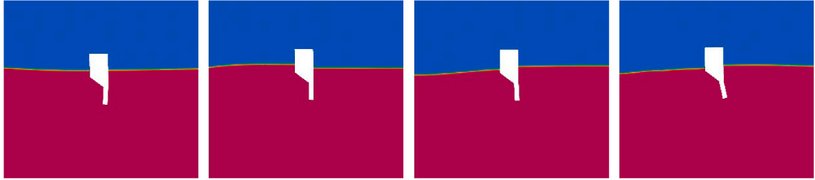
Fig. 10. Simulation example of the HH WEC-breakwater system, (a) t = nT , (b) t = nT + 1/4T , (c) t = nT + 1/2T , (d) t = nT + 3/4T .
