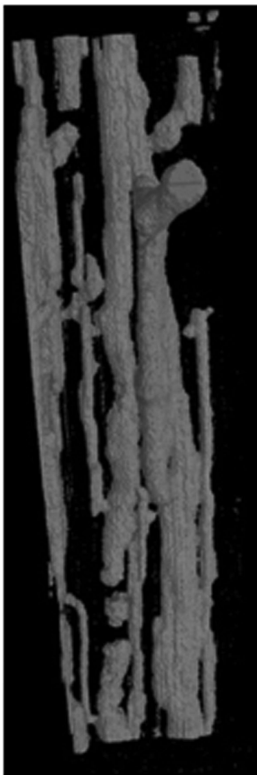
Figure 9. Model of the tunnel voids from Block 6a. Total height of block is ca. 90 mm.
