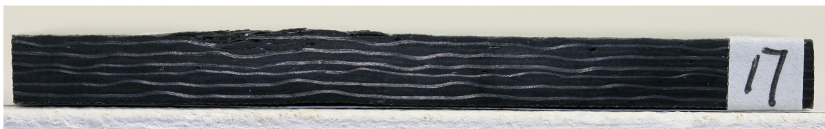
Figure 108 The cross-section of No.17 (5HS woven preform/LY564/veil)
