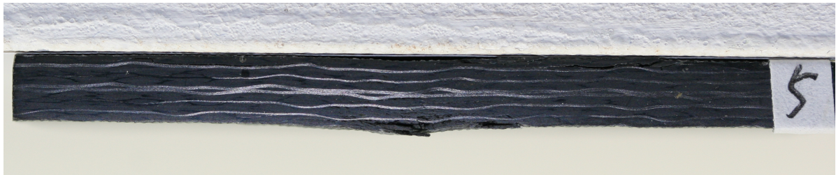
Figure 95 The cross-section of No.5 (5HS woven preform/3508)
