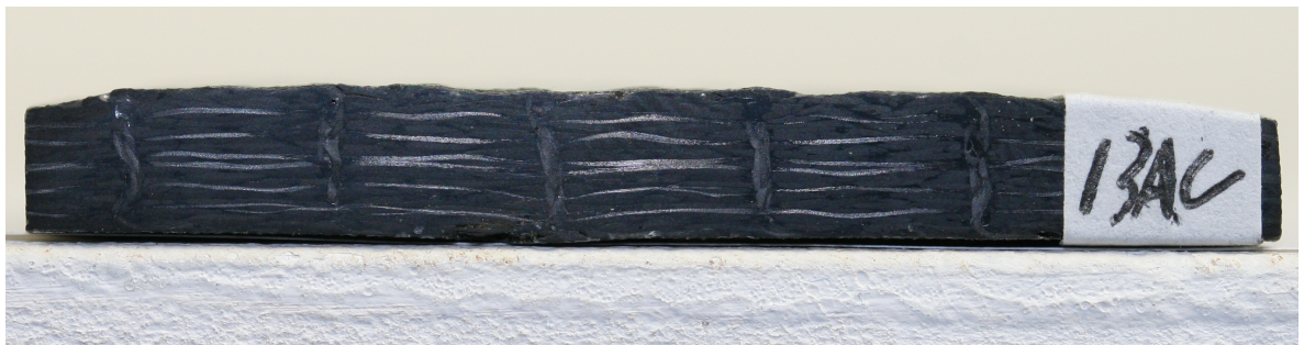
Figure 102 The cross-section of No.13AC (5HS woven preform/LY564/C-tuft)
