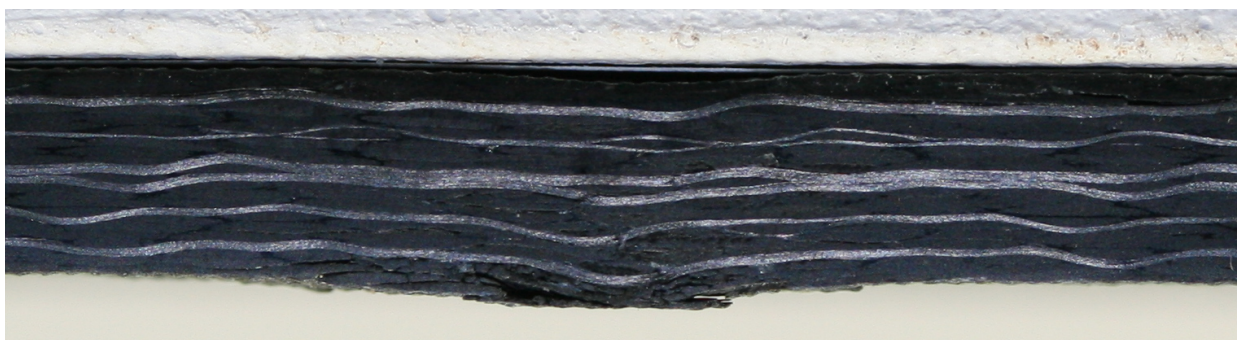
Figure 111 The close-up of the damage inside No.4B (5HS woven preform/RTM6)
