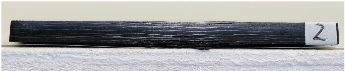
Figure 91 The cross-section of No.2 (T800/M21 Woven Prepreg)
