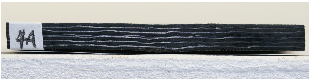
Figure 93 The cross-section of No.4A (5HS woven preform/LY564)
