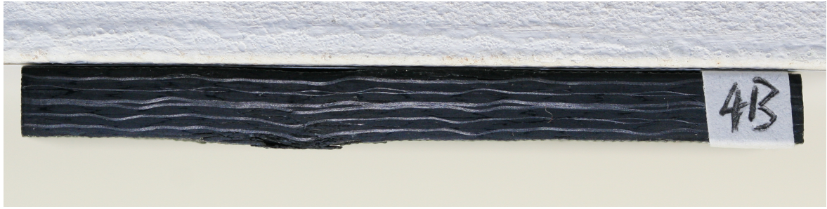
Figure 94 The cross-section of No.4B (5HS woven preform/RTM6)
