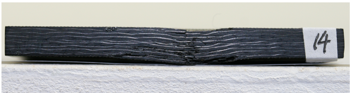
Figure 106 The cross-section of No.14 (T300/913 Woven Prepreg)
