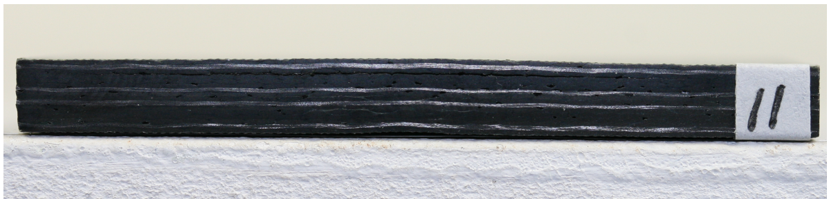
Figure 101 The cross-section of No.11 (uniweave preform/binder/LY564)
