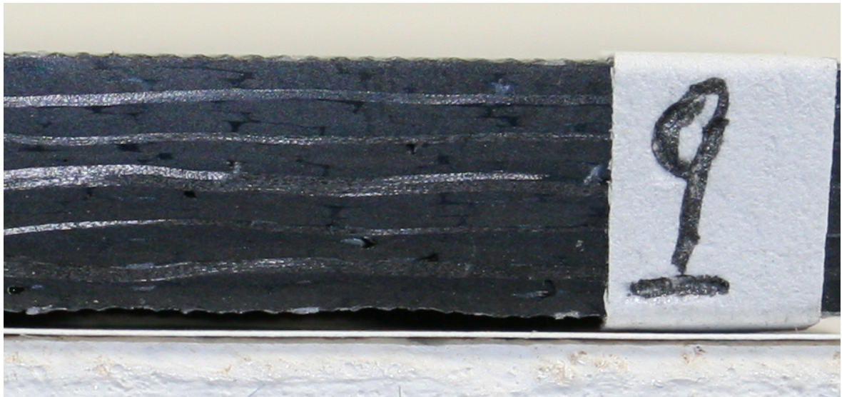
Figure 109 Sporadic, discontinuous, small voids inside of NCF/LY564 panel)
