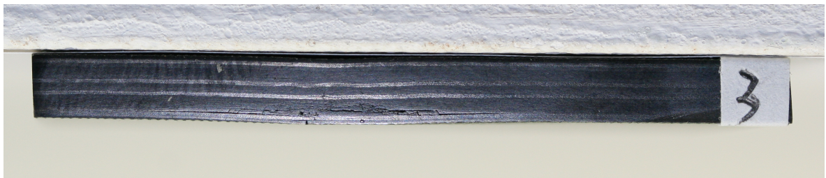
Figure 92 The cross-section of No.3 (T700/M21 UD Prepreg)
