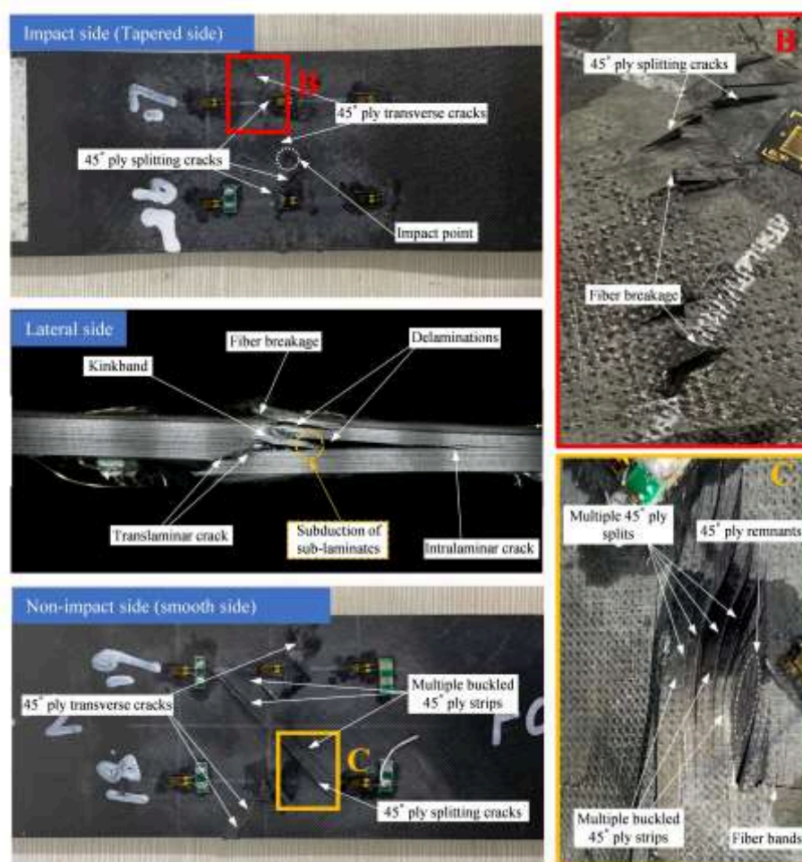
Fig. 21 Damage inspection of the tapered laminate under CAI test (macroscopic visual inspection and microscopic inspection).
