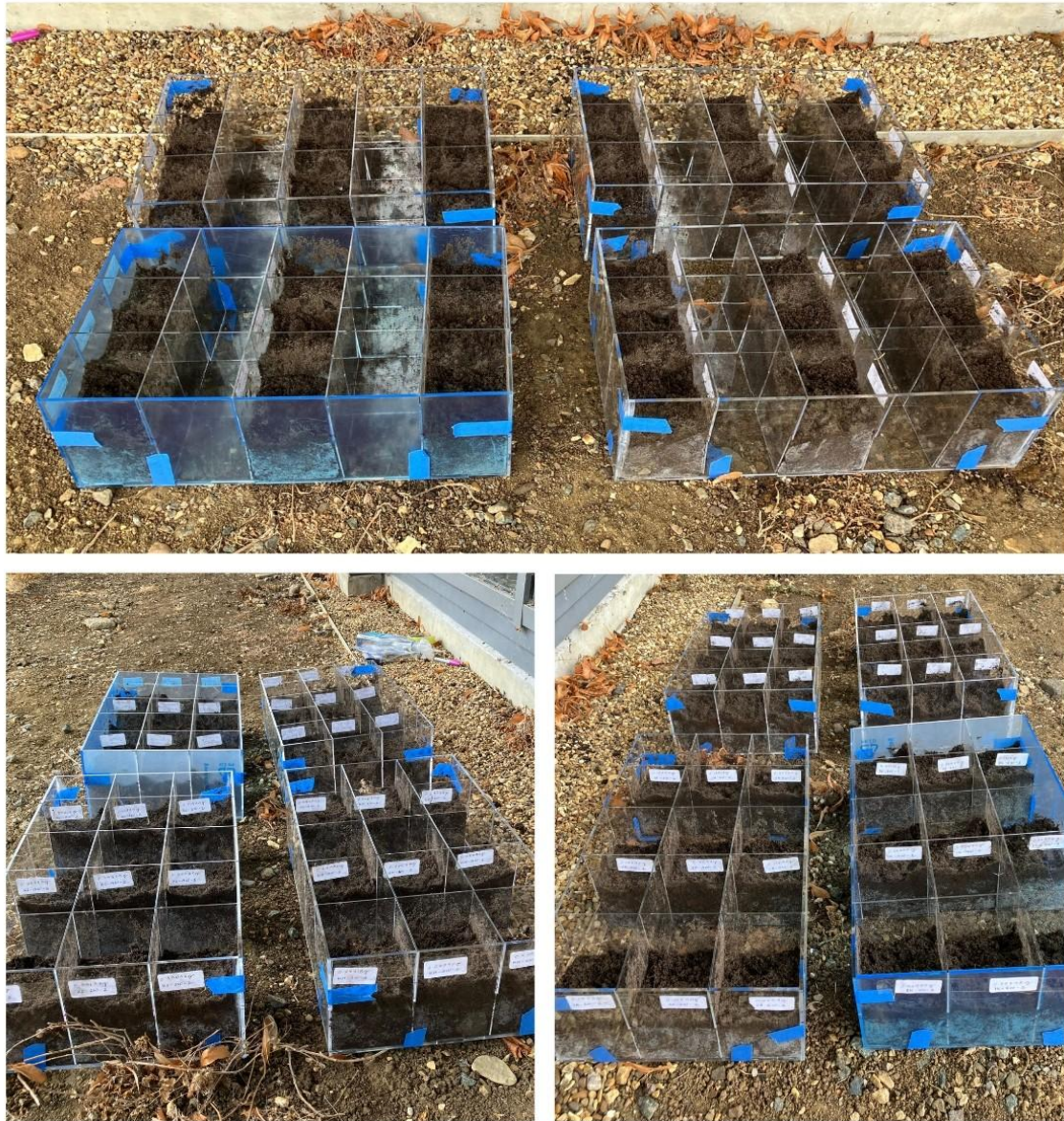
Figure D-7 Soil burial tray setup for ISO 11721-1 biodegradation test. Handloom cotton specimens (Khadi, Kala Cotton, Jamdani, Ikat) were enclosed in nylon mesh bags and buried at 5–10 cm depth in loamy topsoil (pH 6.5, 60–65% water-holding capacity).
