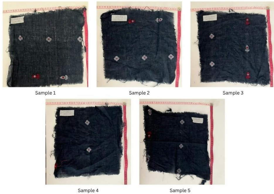
Figure D-5 After-wash specimens of Jamdani following ISO 6330 (40 °C wash cycle)-Quantitative shrinkage data are provided in Appendix C -Tables C-11
