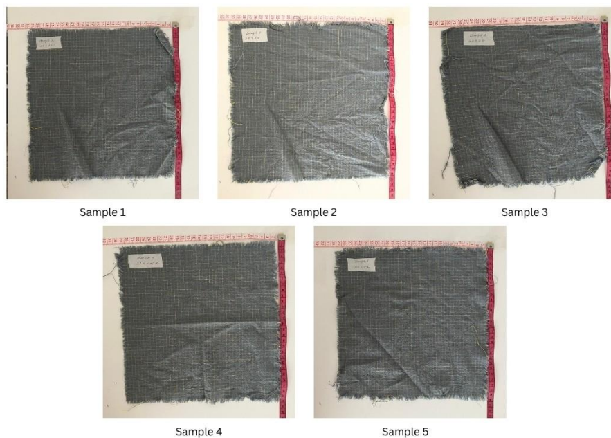
Figure D-4 After-wash specimens of Kala Cotton following ISO 6330 (40 °C wash cycle)- Quantitative shrinkage data are provided in Appendix C -Tables C-10
