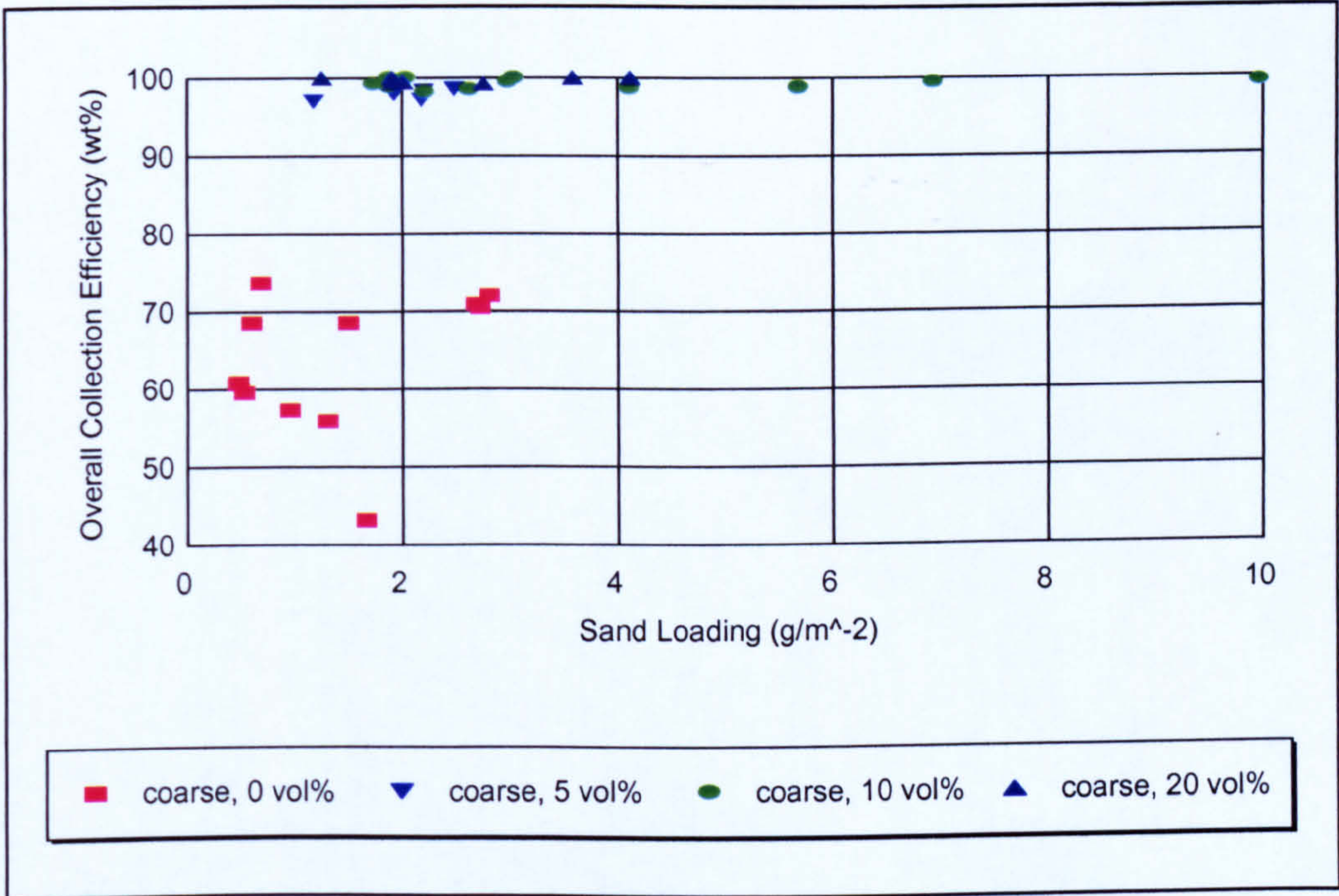
Figure 4.13: Graph showing the effects of different solid loadings ( \text{gm}^{-3} ) on the overall collection efficiency (wt%) for the 'coarse' test sample.
