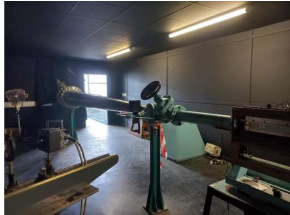
(b) Wind tunnel control valve
