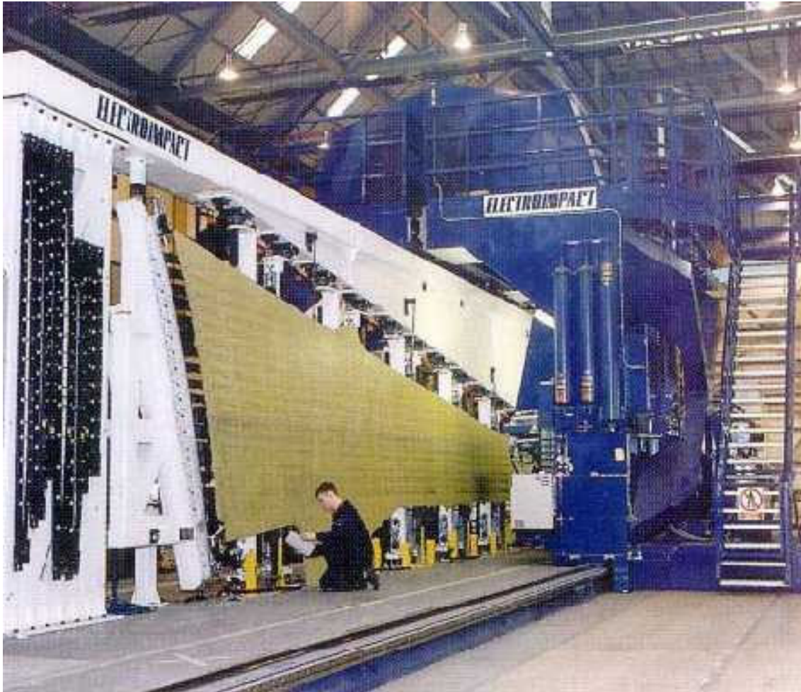
Figure 2.3 Example of an LVER machine (Airbus News, 1999)
