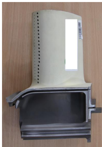
Figure 3-5: Low-pressure-turbine 1 st stage blade
