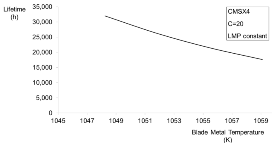
Figure 4-53: Remaining life of CMSX4 over increasing metal temperature
