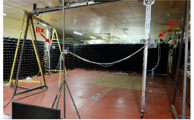
FIGURE 2 The GBSAR laboratory in a bistatic configuration.
