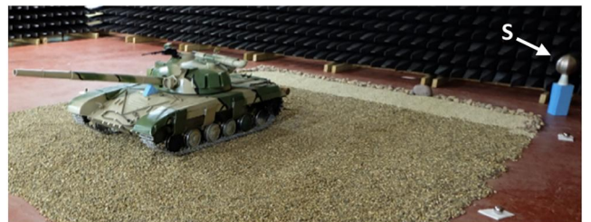
FIGURE 4 Target scene, consisting of a Quarter scale T72 tank model on gravel and reference sphere “S”.
