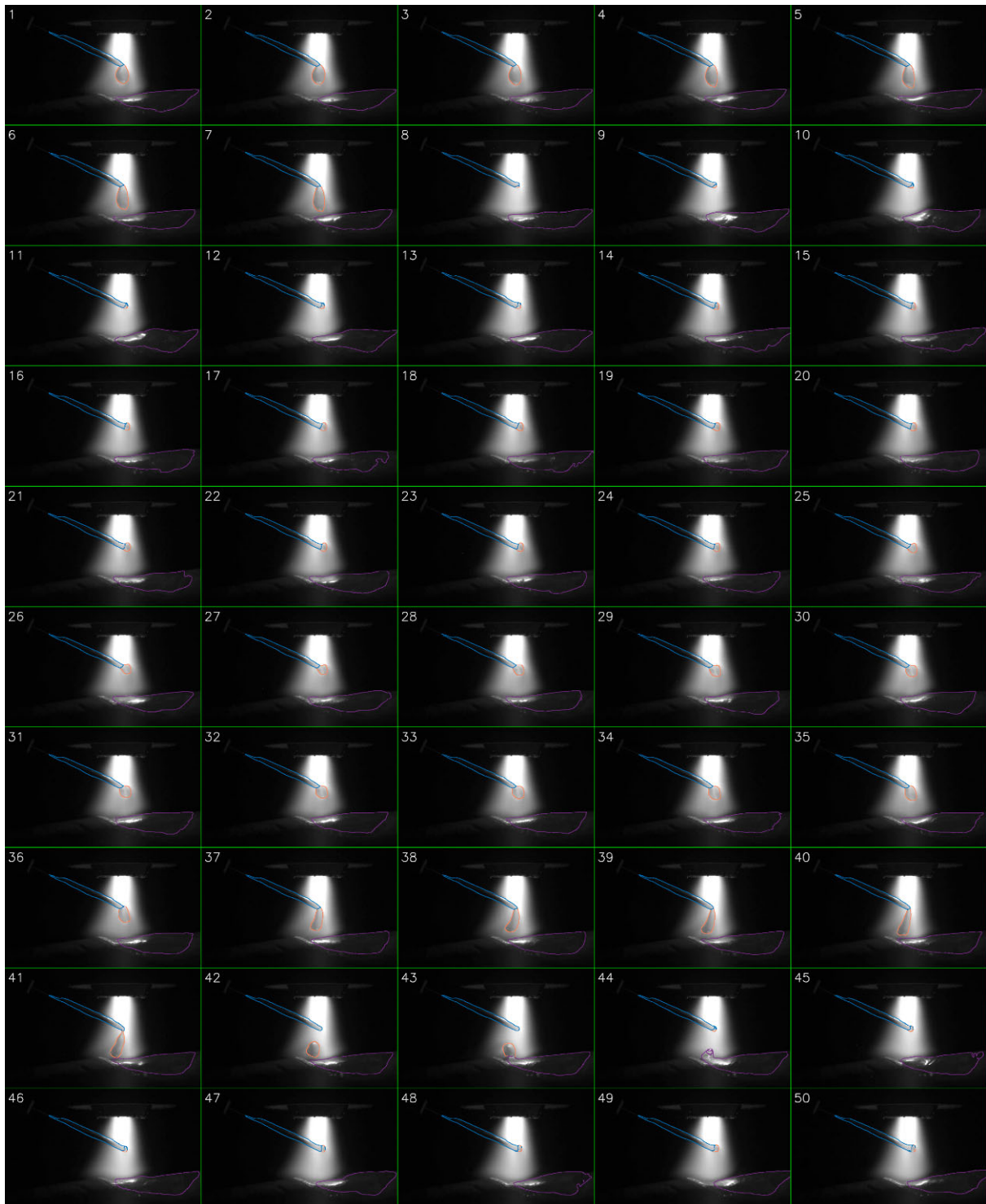
Figure 9. A 50-frame sequence extracted from a segmented plasma WAAM video, showcasing a complete droplet transfer process.
