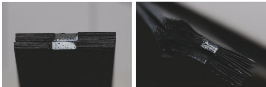
Fig. 4. Representative post-failure fracture patterns in the U-notched laminated composites. Specimens include: a) CP_00_U (brittle, fibre-dominated net section failure), b) CP_45_U (fibre-dominated net section failure along a path perpendicular to the load application direction).
