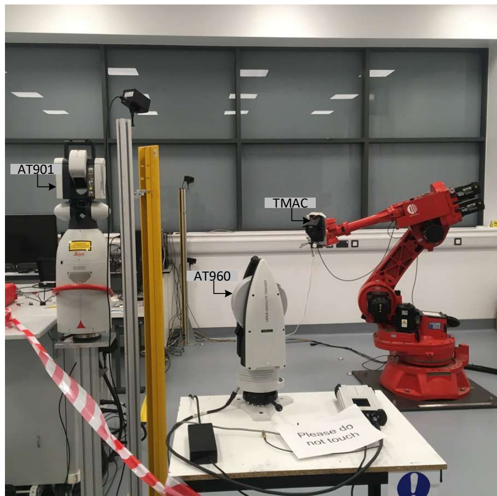
Figure 16. AT960 Leica Tracker Setup for NRTEC Verification.
