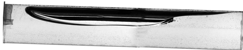
(b) 160cp_0.099m ID pipe_2.5degree, (STT)
