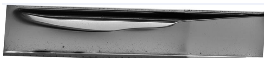
(a) 160cp_0.099m ID pipe_2.5degree_Vso = 0.11m/s
