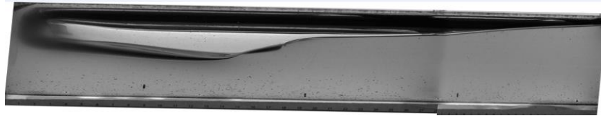
(c) 160cp_0.099m ID pipe_2.5degree_Vso = 0.31m/s
