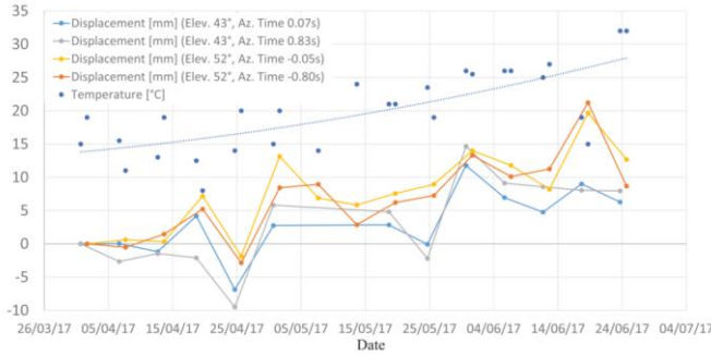
Fig. 13 Displacement time series [mm] of the observed plaza building and the temperatures [°C] at the dates of acquisition [75].
