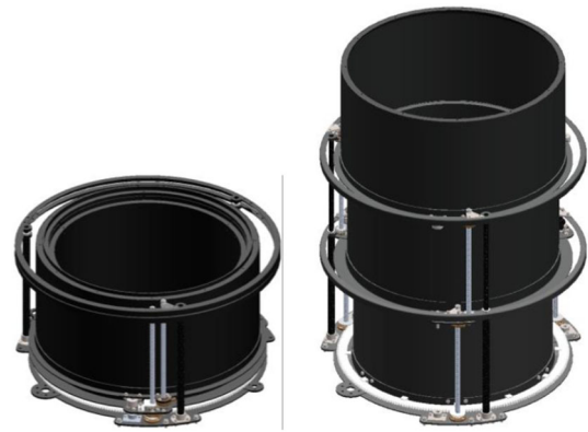
Fig. 1 Telescope structure in stowed and deployed configuration
