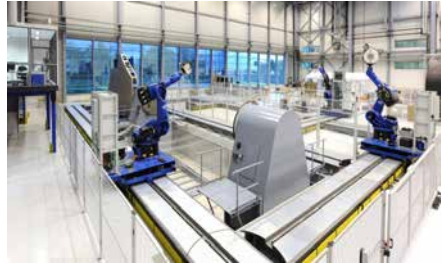
Figure 2: Photo of the automated fibre placement plant GroFi ® at the Center for Lightweight-Production-Technology
