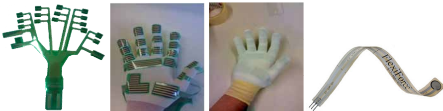
Figure 3: The force sensors used; Gryp system (and the glove with sensors) and the Flexiforce
