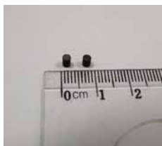
Figure 4: The formed samples (solid cylinder) with a size of \Phi 4.0\text{mm} \times 4.0\text{mm}
