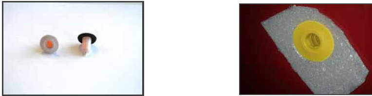
Figure 2: The new plastic bushes (P-pink & Y-yellow) with gasket and water sealing.
