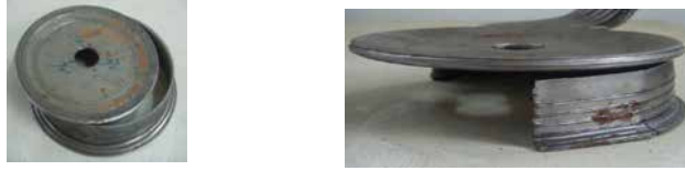
(a) bottom cutting-off during thickening (b) bottom cutting-off during toothing Figure 6: Bottom cutting-off
