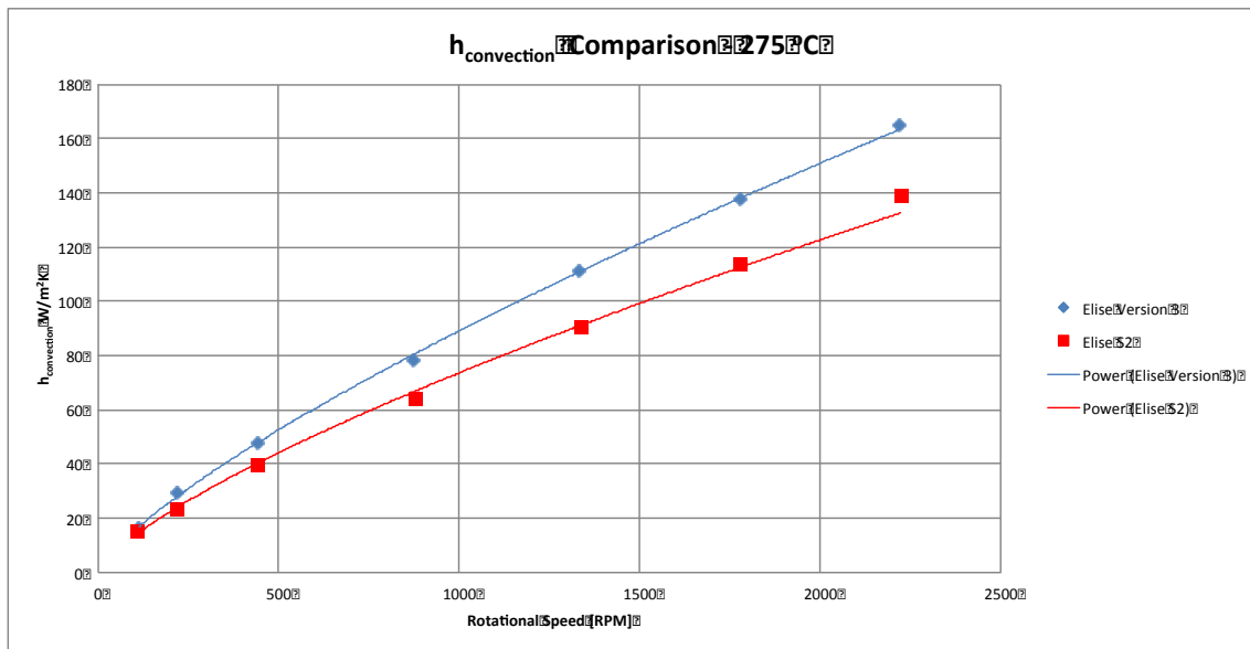
Figure 9-3 Elise Version 3 VS Elise S2 Convective HTC at 275°C
