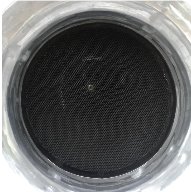
Figure 7-9 Detail of the Flow Straightener Honeycomb
