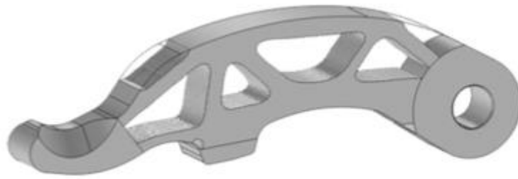
Figure 6-11 Optimised Component with Constant Cross Section (Kumagai, et al., 2016)
