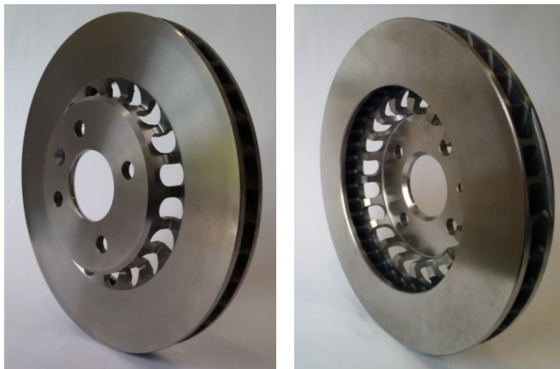
Figure 1-2 Prototype Elise Brake Disc with Fingered Hub
