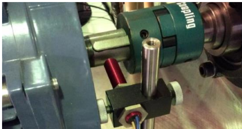
Figure 7-39 Rotational Speed Hall Sensor Installation
