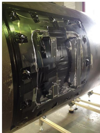
Figure 9-10 Sealing the Hatch Doors (Disc Rotating and Heating Assembly not in the Picture)
