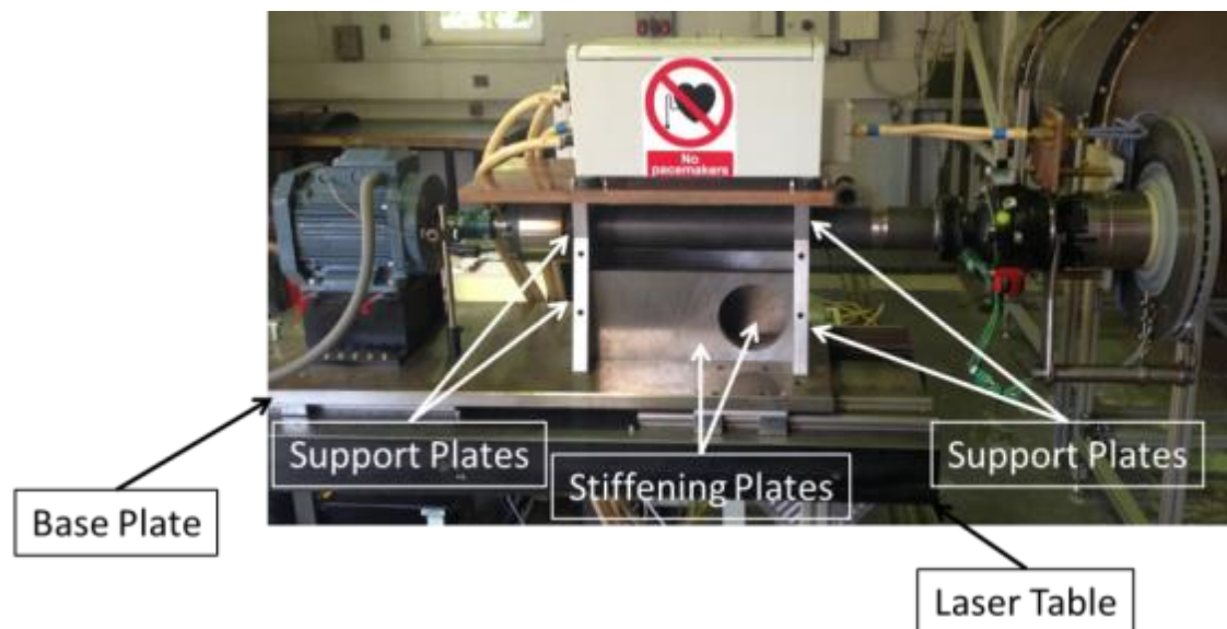
Figure 7-23 Support and Stiffening Plates
