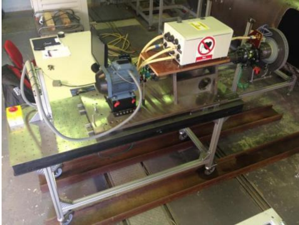
Figure 7-18 Disc Rotating and Heating Assembly Table
