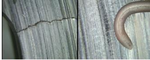
Figure 2-17 Left: Sudden Crack in a Non-bedded Disc Early in its Life, Right: Acceptable Microcracks During a Discs' Service Life (Mace, et al., 2006)
