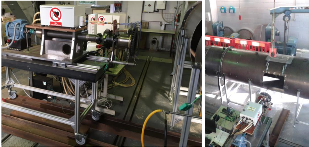
Figure 9-2 Elise Version 3 Disc Ready to be Tested in Still Air
