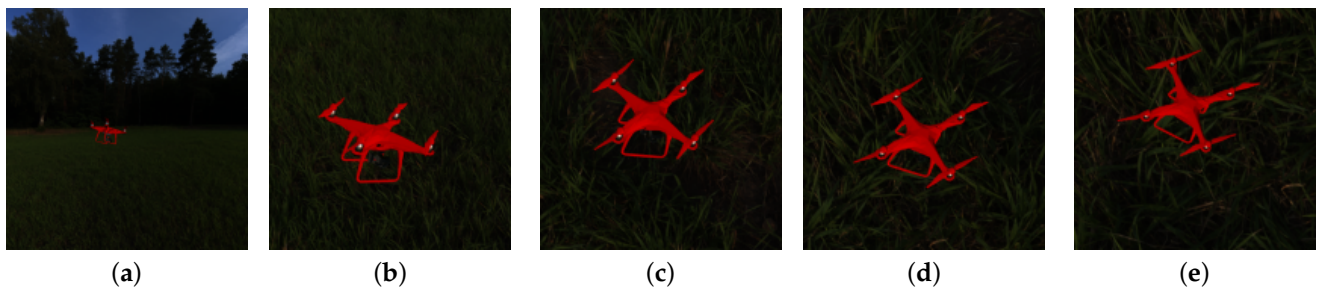
Figure 10. Viewport from the camera at (a) frame 1, (b) frame 75, (c) frame 150, (d) frame 225, (e) frame 300 during an episode of the basic tracking scenario. The agent correctly tracks the drone for the entire 300 frames in this episode.
