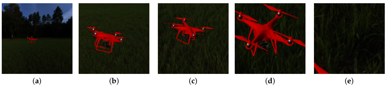
Figure 15. Viewport from the camera at (a) frame 1, (b) frame 75, (c) frame 150, (d) frame 250, (e) frame 286 during an episode of the Dynamic Tracking B scenario. The agent correctly tracks the drone for most of the frames but the drone leaves the viewport in frame 287 in this episode.
