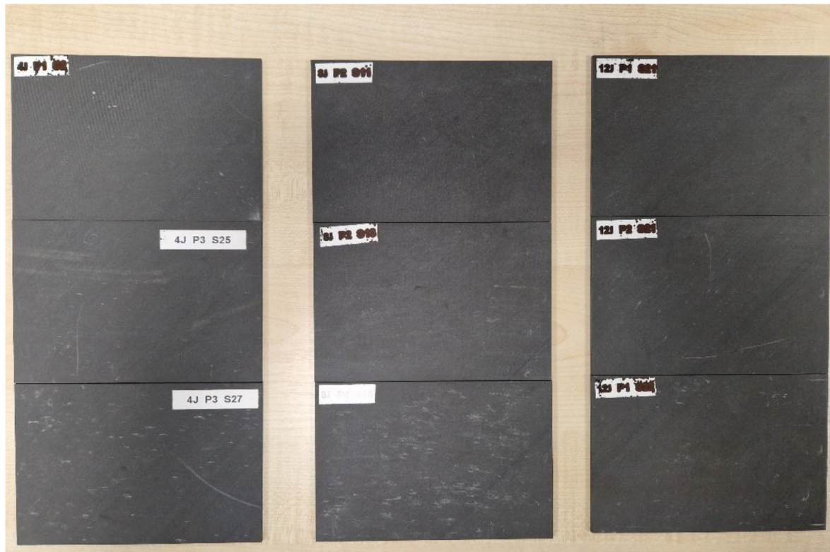
Fig. 5. CFRP samples that have undergone impact damage at energies of 4J (left) 8J (middle) and 12J (right).
