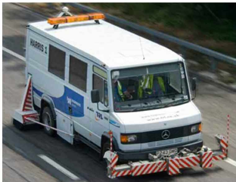
Fig. 1. Traffic speed survey vehicle HARRIS1, showing laser bar on the front used to make measurements of surface texture via the deflection of projected laser beams. Taken from 4 .
