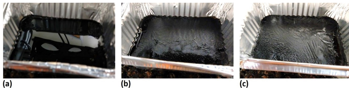
Fig. 10. Examples of (a) fresh, (b) 2-week, and (c) 5-week UV-aged bitumen.
