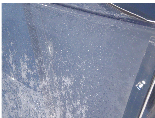
FIGURE 4.8: Shielded CR with a ice layer on top of the shield.
