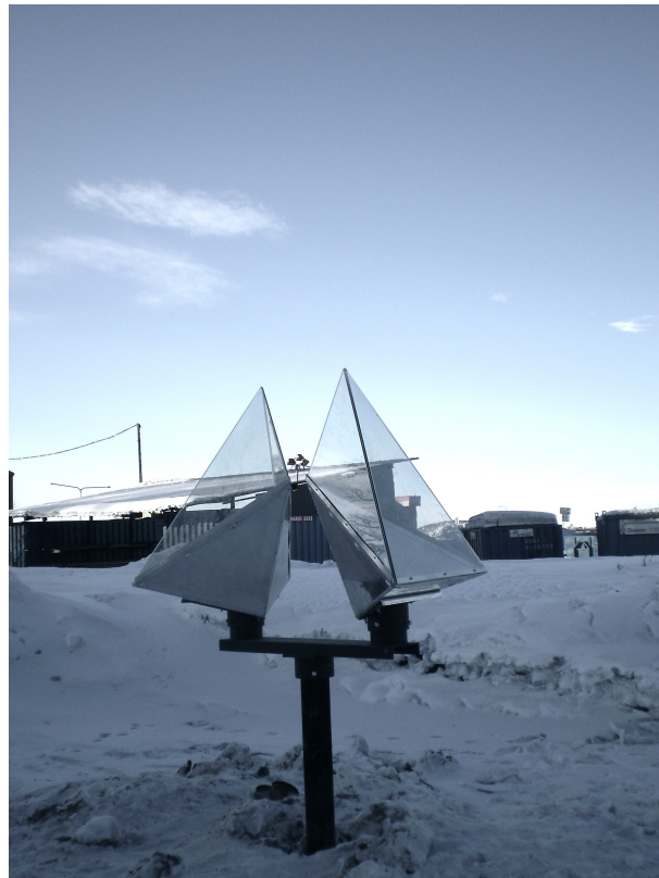
FIGURE 4.6: Shielded CR installed in Kiruna without snow.
