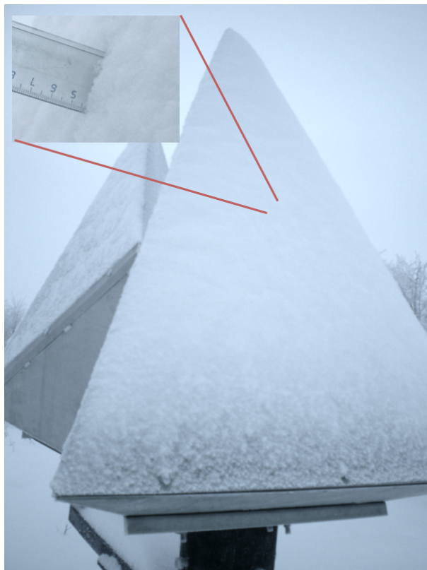
FIGURE 4.7: Shielded CR with a snow layer on top of the shield.
