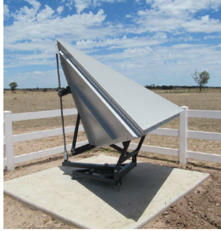
FIGURE 2.9: A corner reflector installed in the field [66]
