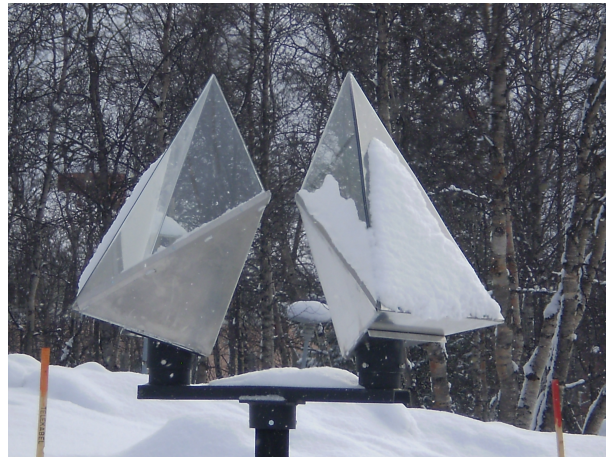
FIGURE 4.9: CR with inhomogeneous snow cover on top of the shield; some of the snow has been blown off by wind.
