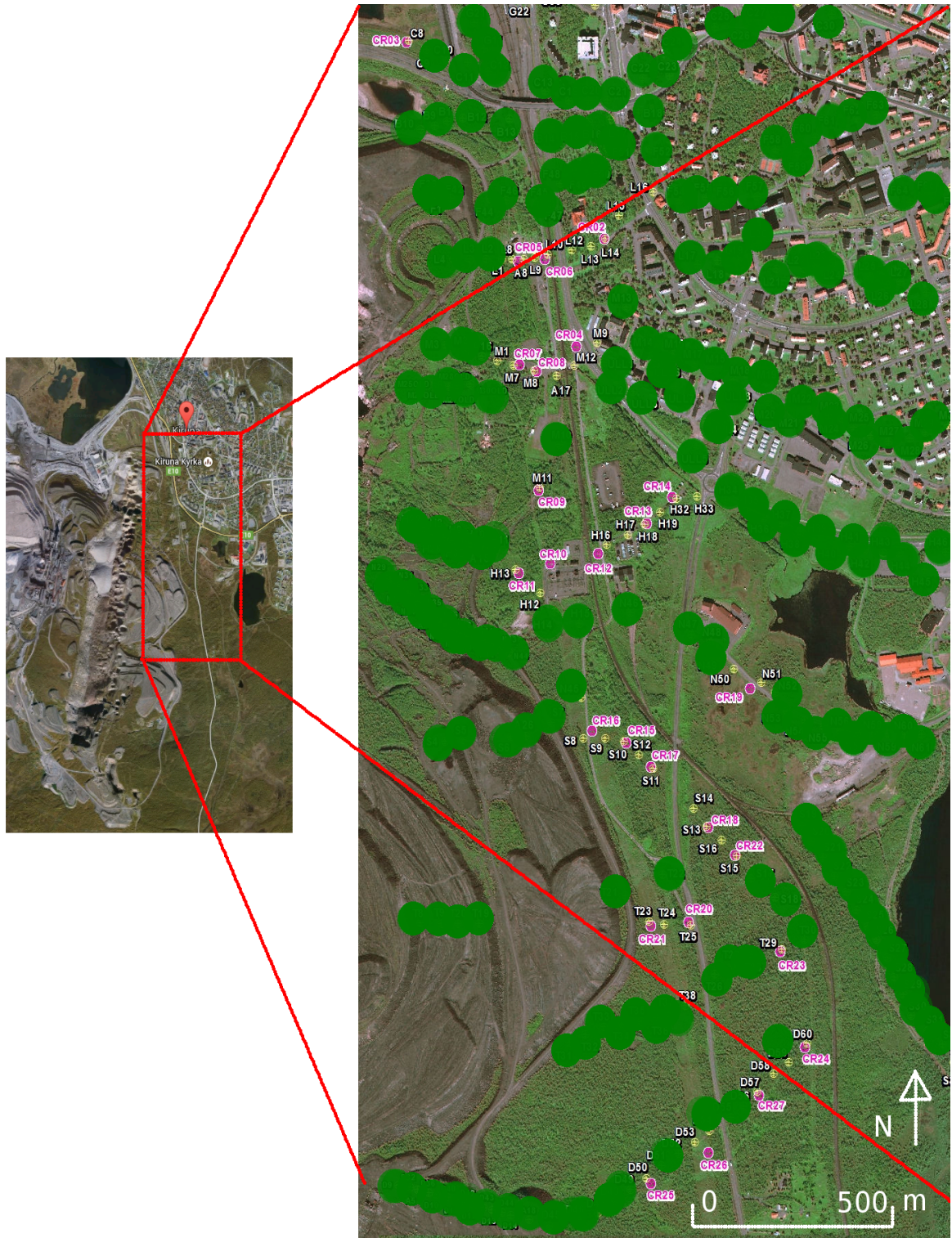
FIGURE 4.1: GPS and CR network in Kiruna. The red box in the left image shows the general area where corner reflectors are installed. Right image shows the CR installed area in high resolution. CRs are marked in purple, and GPS measurement points are marked in yellow. Selected areas of the image are masked out to protect LKAB proprietary information (image source: LKAB and Google maps).
