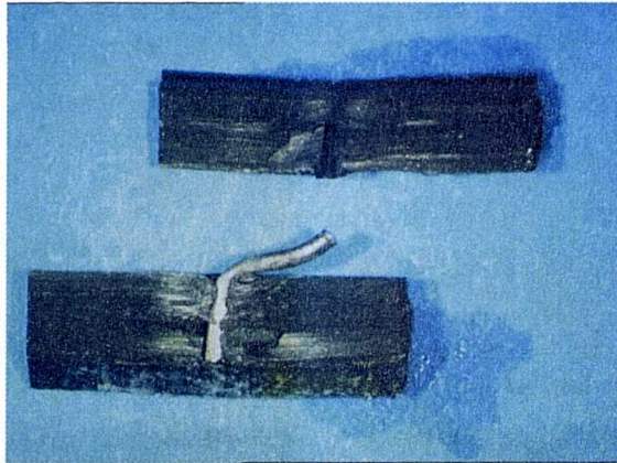
Figure 6-21: Titanium Z-Fibre in shear in the nap (No opening displacement)
