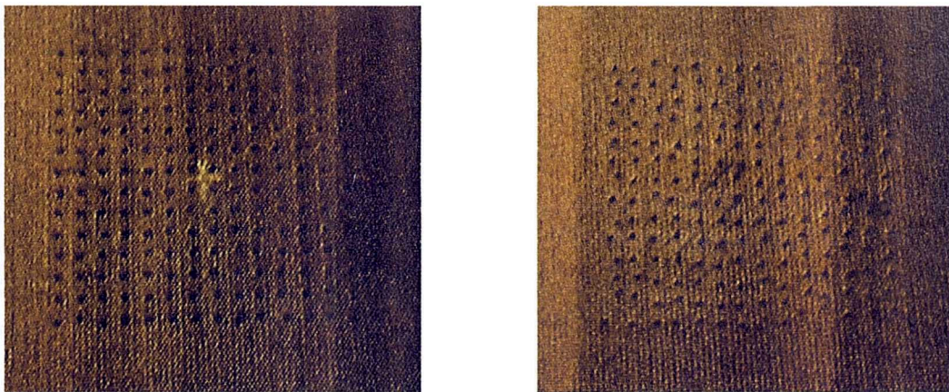
Figure 8-11: Top and bottom surface of a 2%-0.28mm pinned CAI specimens (Sample by courtesy of Bitsianis, 1999)
