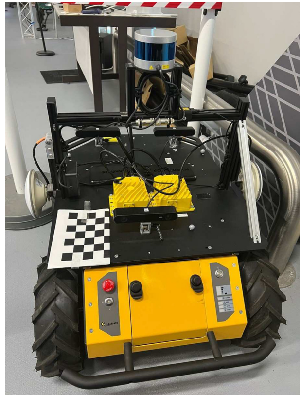
Fig. 16. Husky A200 Vehicle Platform snapshot with VLP 16 Lidar, Stereo Camera, Duro RTK GPS sensors payload (Centre for Autonomous & Cyber-Physical Systems, Ground autonomy Lab, Cranfield University).
