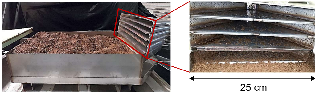
Figure 3-5 The erosion tray with a set of collectors downslope collecting the detached soil particles by rainsplash due to windless and wind-driven rains.
