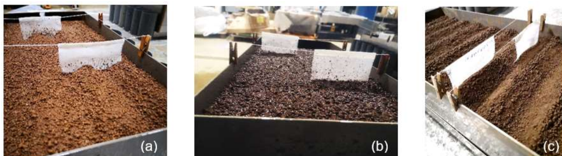
Figure 2-3 Capturing soil particles detached by rainsplash on the erosion trays. (a) Collector voiles cut to fit the shape of Treatment A. (b) Two collector voiles placed at the top and bottom of the erosion tray. (c) Two collector voiles put on the ridge and in the furrow of Treatment B.
