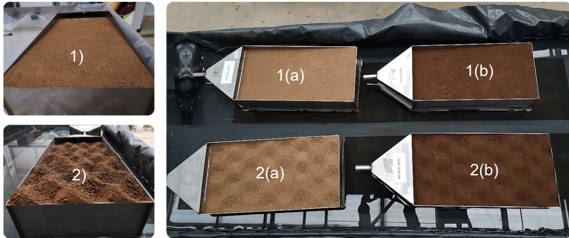
Figure 3-1 Two soil surface conditions applied to a sandy loam soil in erosion trays put in a water bath: 1) smooth surface (a) before wetting up, (b) after wetting up; 2) rough surface with mounds and depressions (a) before wetting up, (b) after wetting up.
