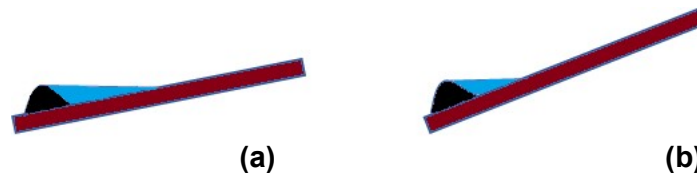
Figure 5-1 Surface storage capacity behind contour features on a gentle slope (a) and on a steep slope (b). Stored water illustrated in blue
