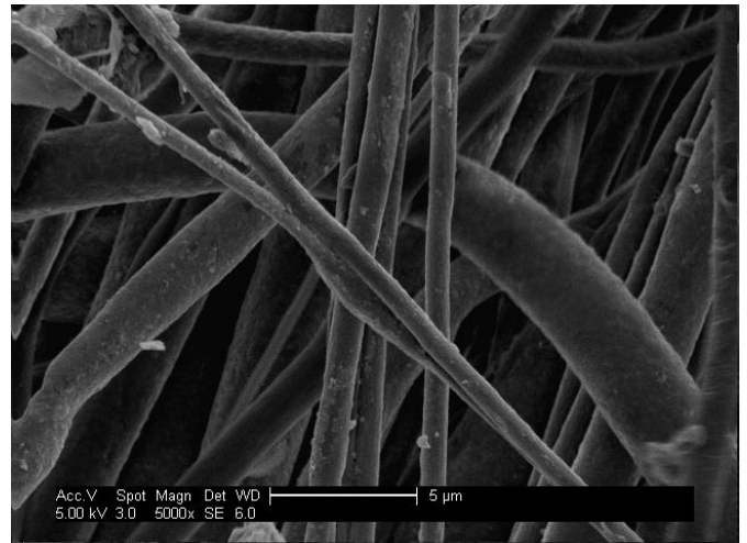
Figure 1: Comparison of morphology of (a) nylon 6, 6 powder and (b) electrospun nanofibers, stretched up to 300%
