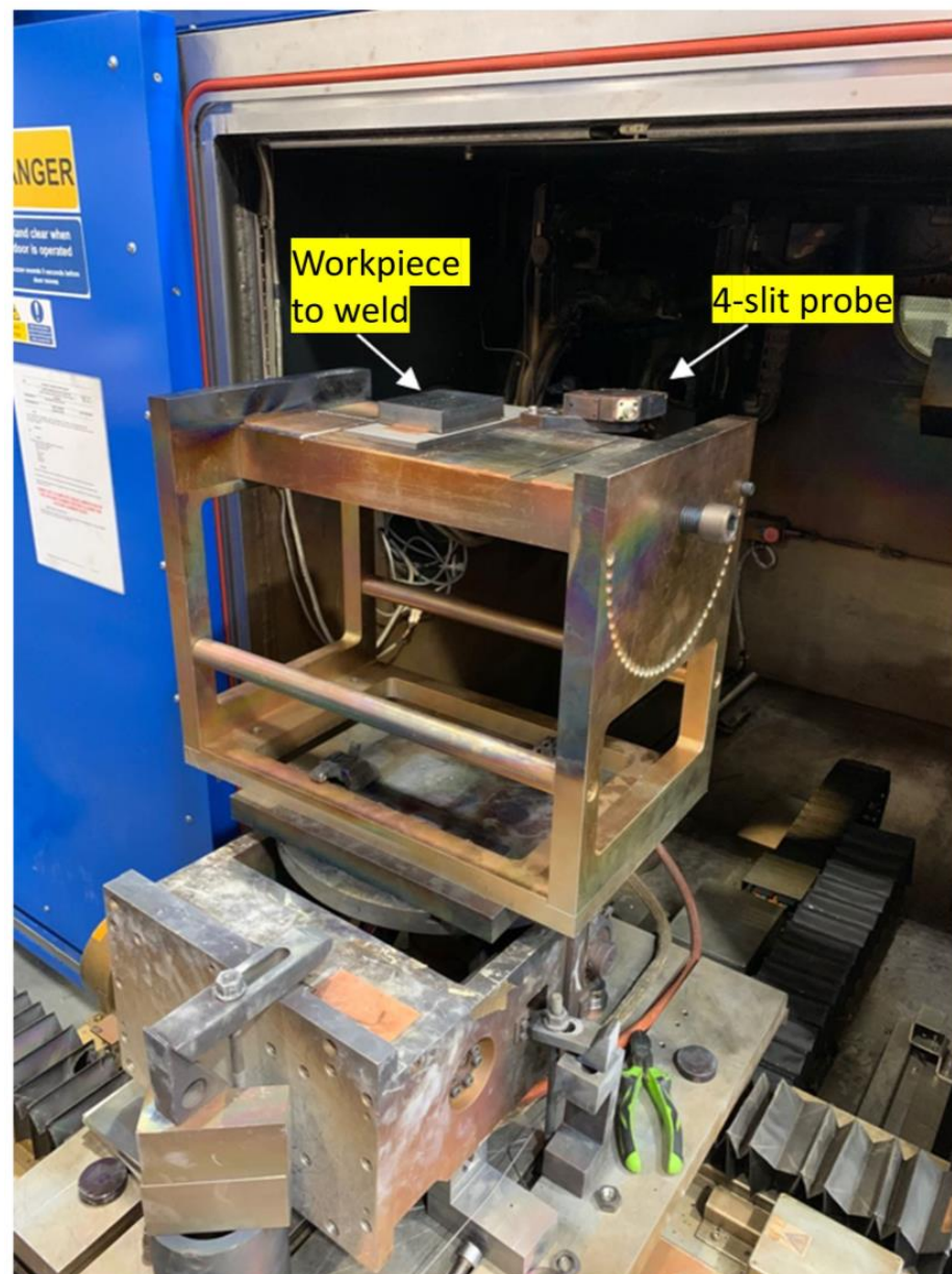
Figure 3. An example of placement of a workpiece to weld and the 4-slit probe.
