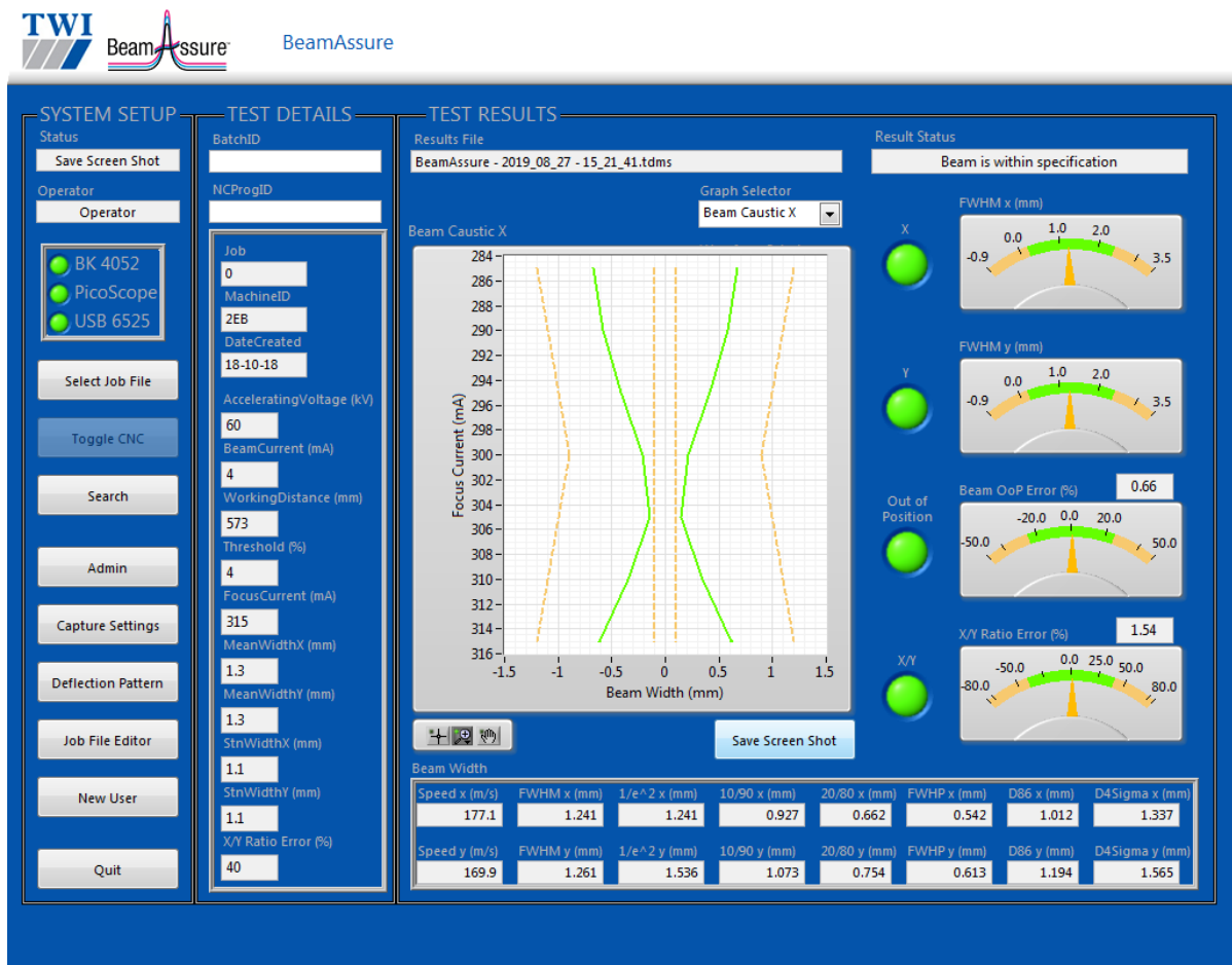
Figure 5. User interface of BeamAssure™ electron beam characterising system. Yellow dashed lines represent the predefined beam radii range, while the green lines represent the actually detected beam radii.
