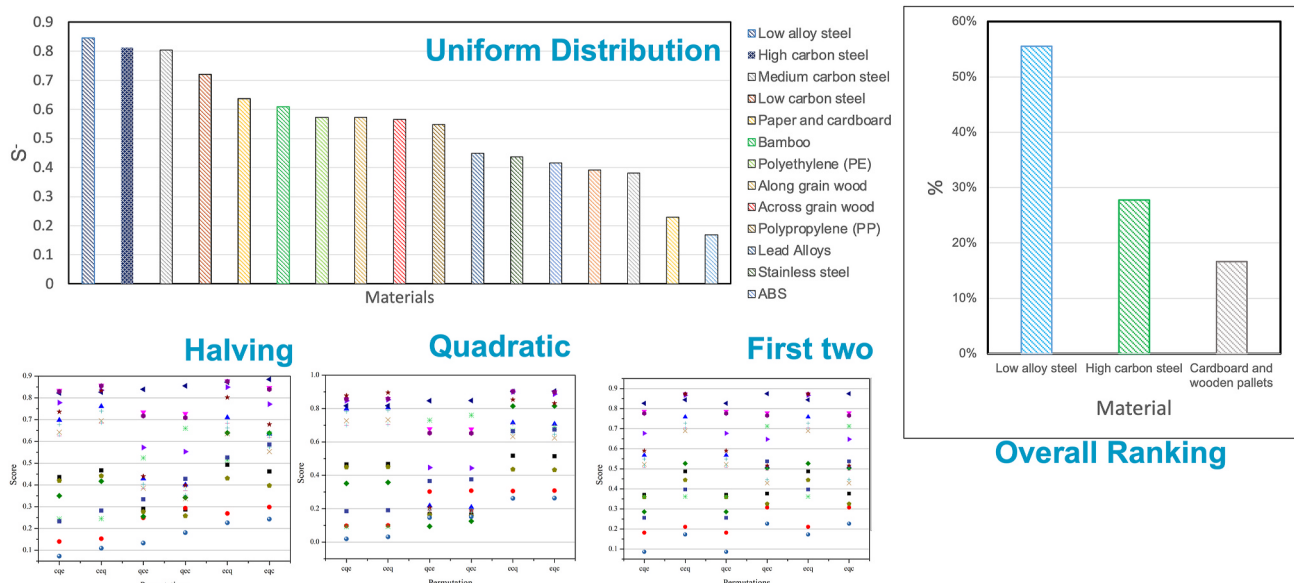
Fig. 12. Dashboard displaying results from all four rules of Automatically Weighted MCDA with an overall ranking of materials for pallets.
