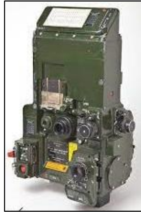
Figure 30 – TLS No 7, Laser Rangefinder, fitted to Chieftain MBT.
