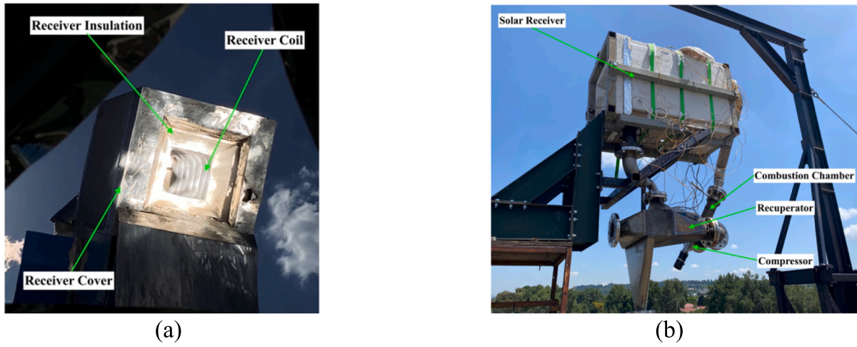
Fig. 4. Insulated tubular cavity solar receiver (a) in operation with cover and (b) during installation without cover.
