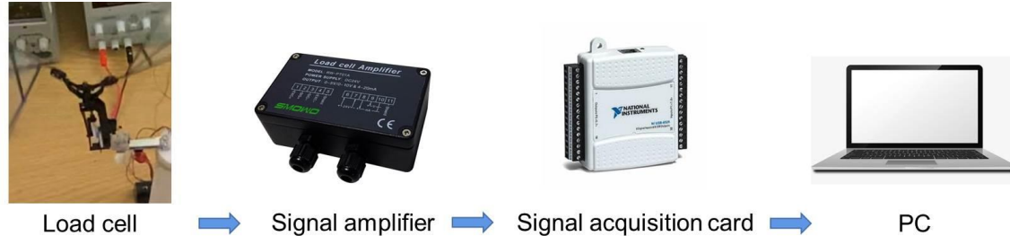
Figure 5-6 The experiment setup for force measurement of FWR wings.
