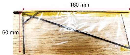
Figure 5-11 Structure and dimensions of Wing RW-C.
