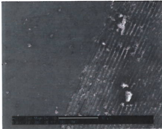
Figure 5: Biofilm formation on the structured surface following 1 week incubation
