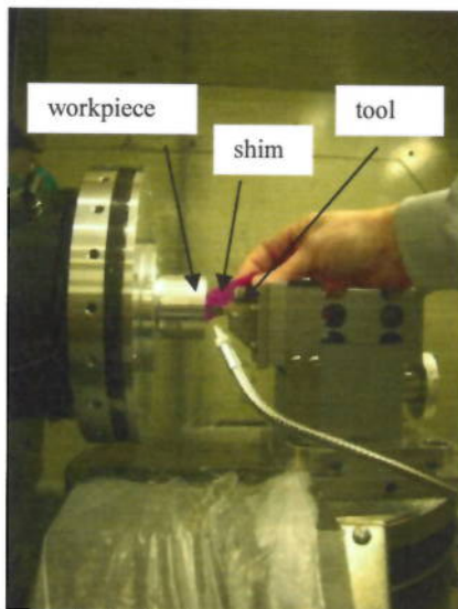
Figure 1: Tool setting on Z axis using a shim.
