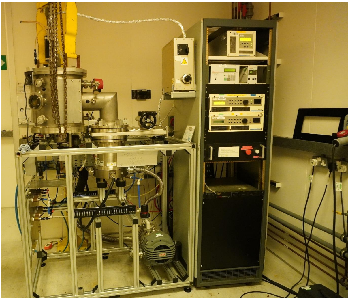
Figure 3-1 Physical Vapour Deposition instrument for the fabrication of the ceramic samples with DC and RF power supply.
