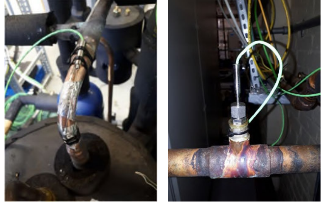
Figure 5: NARROW THERMOCOUPLE (Ø0.75MM) FOR SURFACE MEASUREMENT BEFORE BEING COVERED WITH PIPE LAGGING (LEFT) THERMOCOUPLE INSERTED WITHIN THE PIPE (RIGHT).
