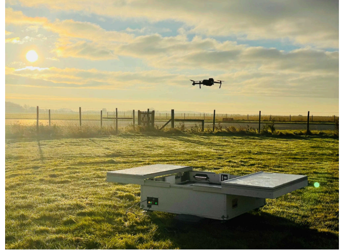
Fig. 1. Autonomous quadrotor hovering above its ground/charging station
