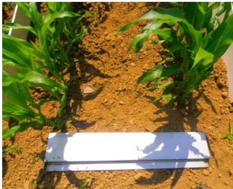
Figure 6 Particular of the Gerlach trough used to collect runoff during the experiments.
