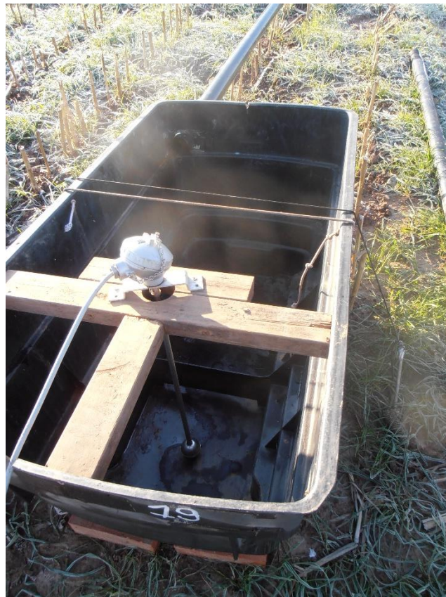
Figure 8 Particular of the linear level sensor land of the ground anchor use to stabilise the tanks during Experiment 2.
