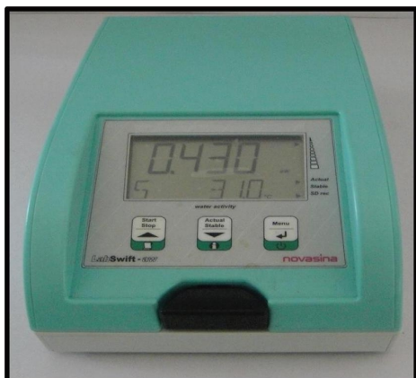
FIGURE 3: Water activity meter.
