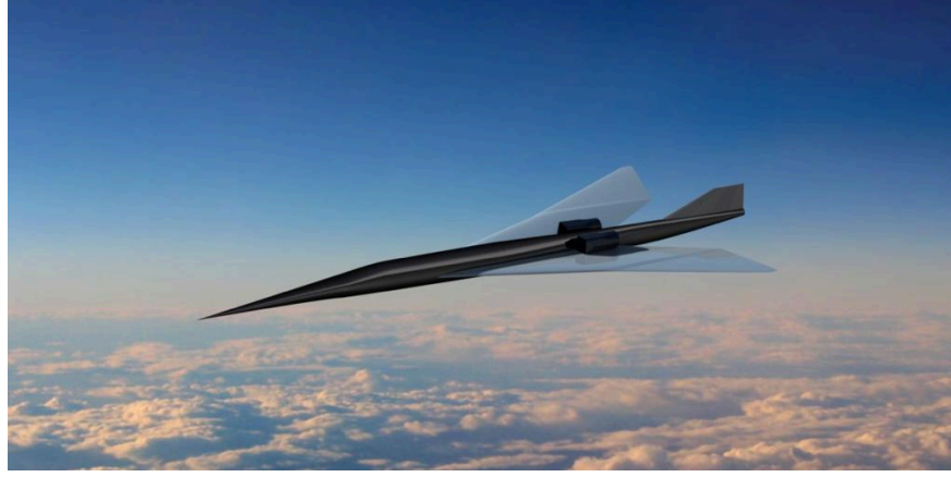
Fig. 2 Baseline aircraft configuration with bell-shaped lift distribution wing.
