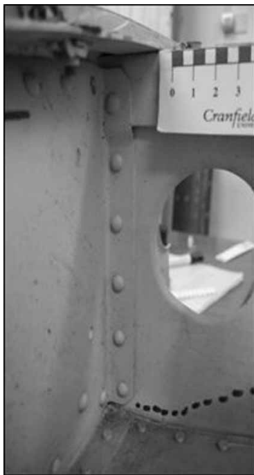
Fig. 13 A lack of intersection joint collapse is a common feature observed during a water impact, as the intersection between STN370A and V0 orientated normal to the water surface demonstrates
