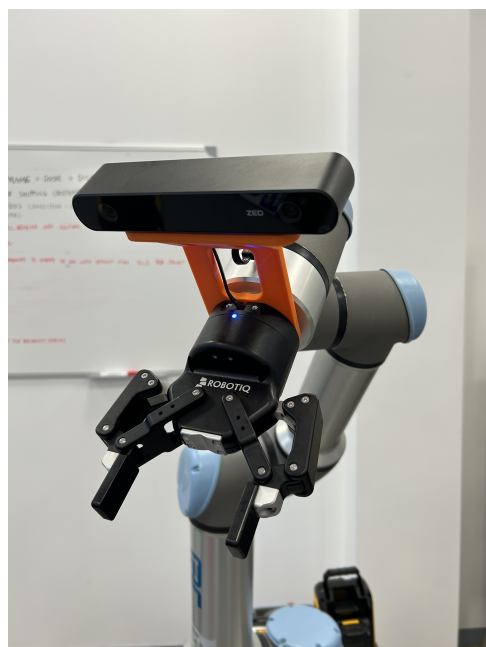
Figure 3. Eye-in-hand ZED 2i stereo camera paired with a Robotiq 2F-85 gripper.
