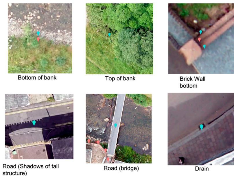
Figure 10. Examples of features where outliers are identified for both S1 and S2. Blue markers indicate outliers. Pink markers are points which fell within the interquartile range.
